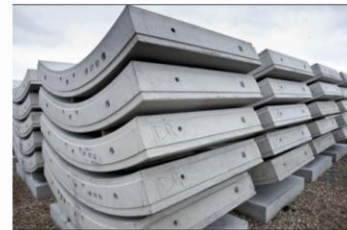
Tunnel Segments (Road and water structures)
